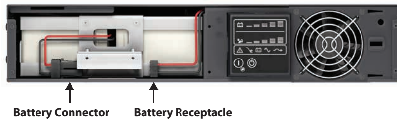
Figure 29: Disconnecting the battery connector and receptacle (front view)
